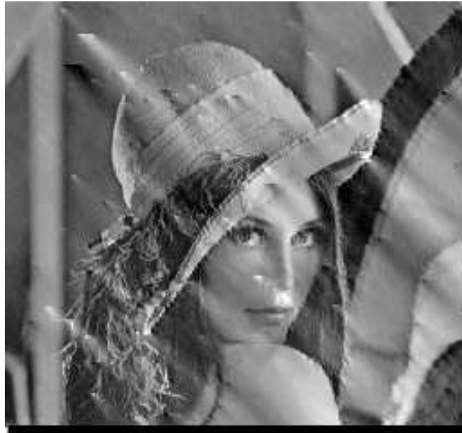
Figure 14: Reconstructed image with an error-prone channel, scalar DPCM algorithm, \text{ber} = 1000
